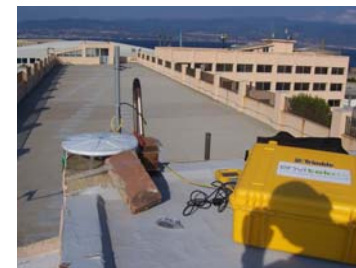
POSITIONING OF GPS RECEIVER ON DATUM POINT
