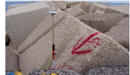
POSITIONING OF "MASTER" GPS RECEIVER ON DATUM POINT
