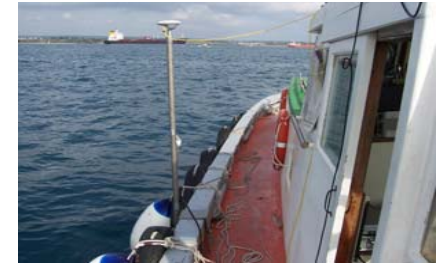
POSITIONING OF "ROVER" GPS RECEIVER ON BOAT
