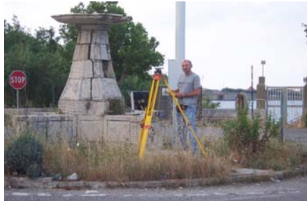
POSITIONING OF GPS RECEIVER ON DATUM POINT
