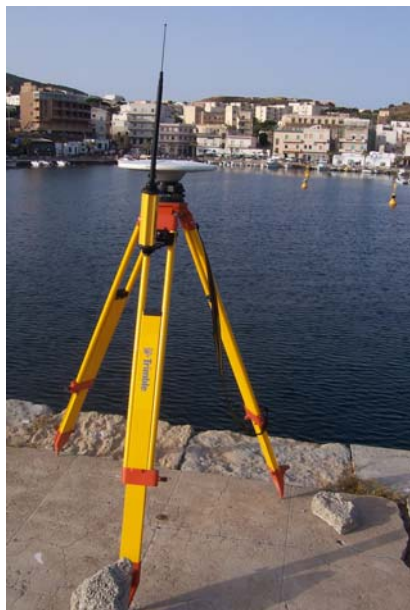
POSITIONING OF GPS RECEIVER ON DATUM POINT
